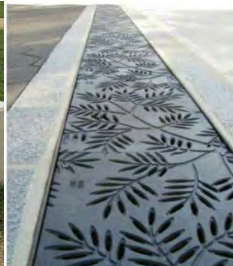
TRENCH DRAIN WITH GRATE - MFR: WWW.IRONAGEGRATES.COM - MODE: LOCUST - FINISH: ALUMINUM - WIDTH: 4" - NOTE RADIAL GRATE AT COMMUNITY ROOM COURTYARD - CHANNEL: CIP CONCRETE, SLOPED TO DRAIN
