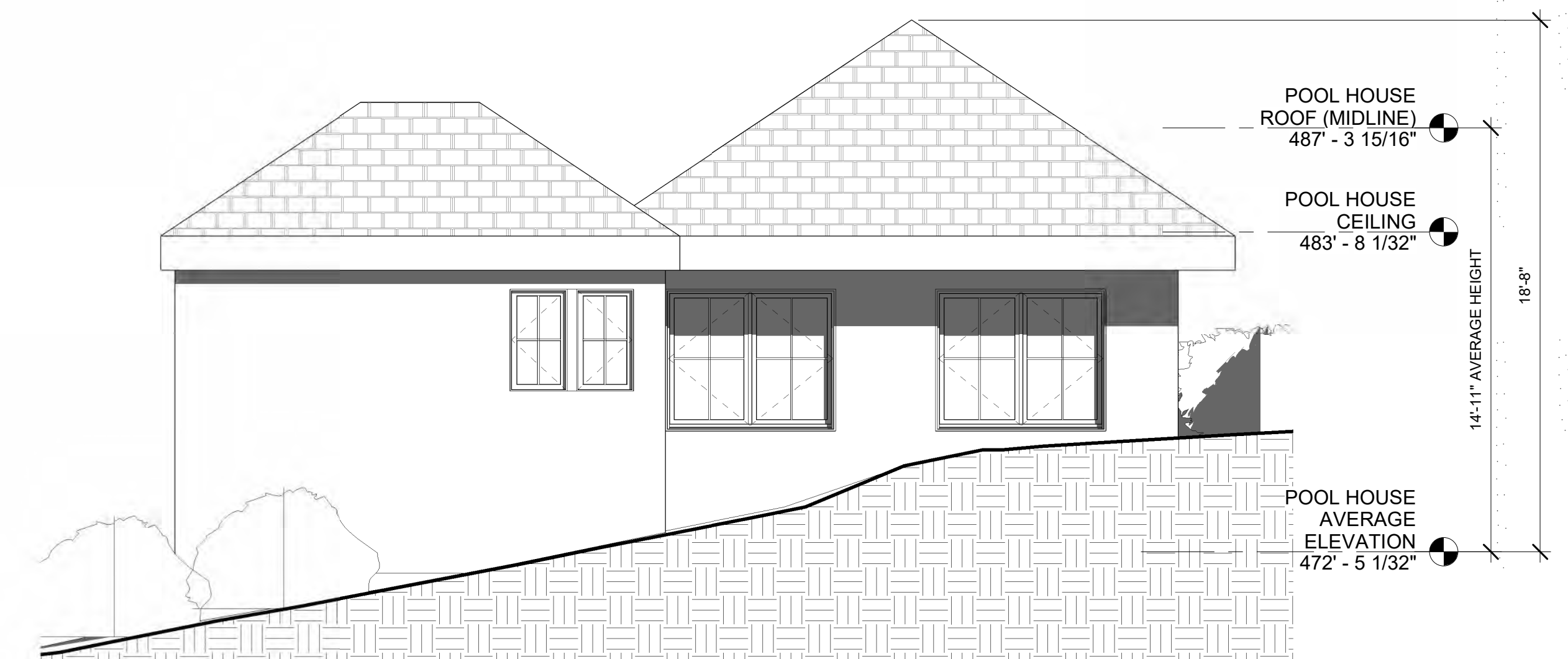
4 POOL HOUSE - WEST ELEVATION 1/4" = 1'-0"
