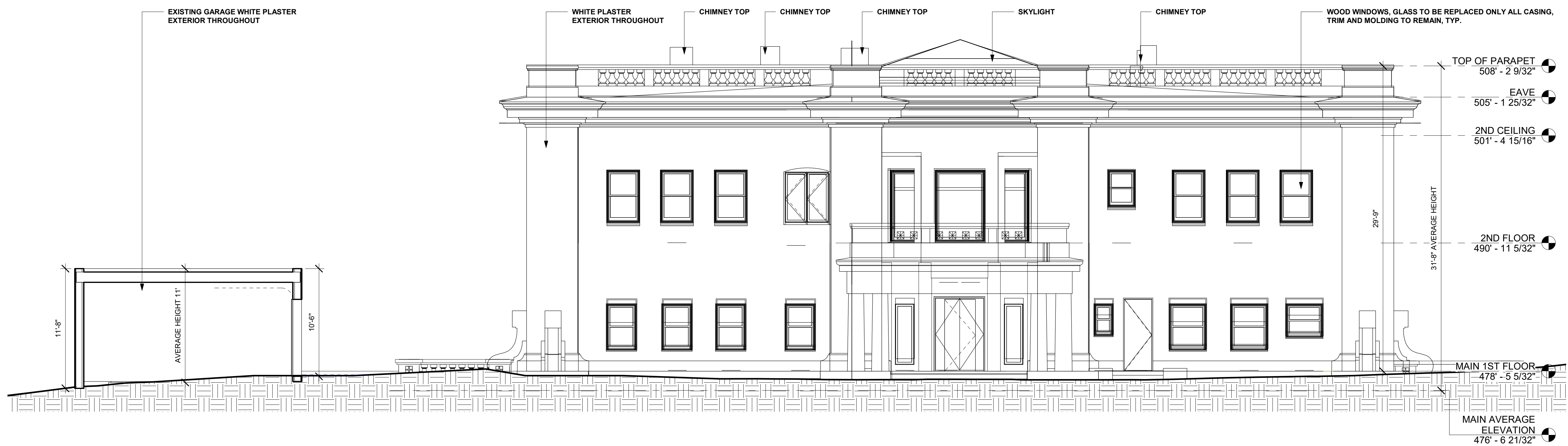
① EAST ELEVATION EXISTING 3/16" = 1'-0"
